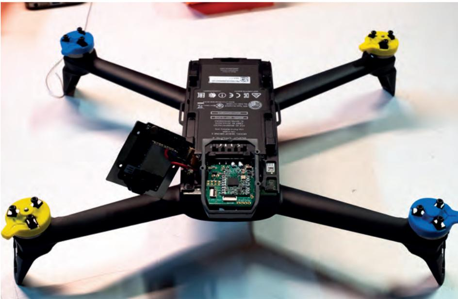
A secondary processor provides for battery management, integrity checks of the main processor and cut-offs of battery power in extreme circumstances
